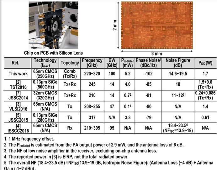
Figure 17.6.6: Die micrograph and performance comparison table.
