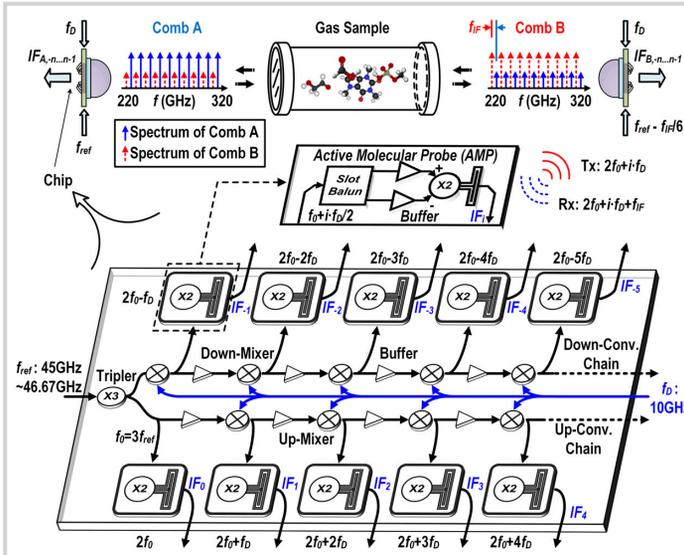
Figure 17.6.1: Dual-frequency-comb spectrometer in CMOS.
