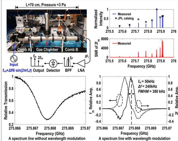
Figure 17.6.5: Spectroscopy for molecular sensing.
