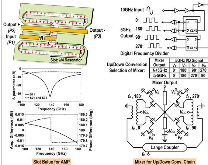
Figure 17.6.3: Slot balun and up/down-conversion mixer.
