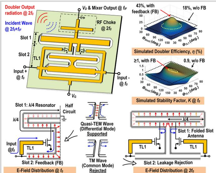
Figure 17.6.2: Active-molecular-probe (AMP) block.
