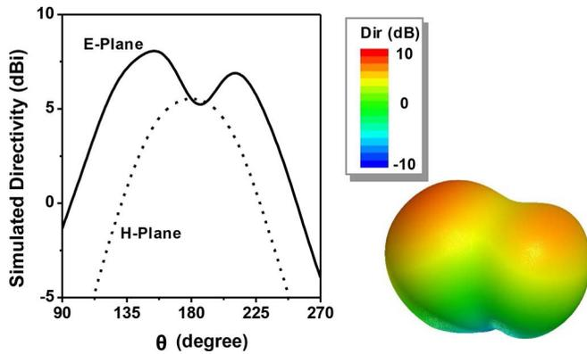
Fig. 13. The simulated radiation pattern of the proposed 320 GHz radiator unit. A backside hemispheric silicon lens is assumed.
