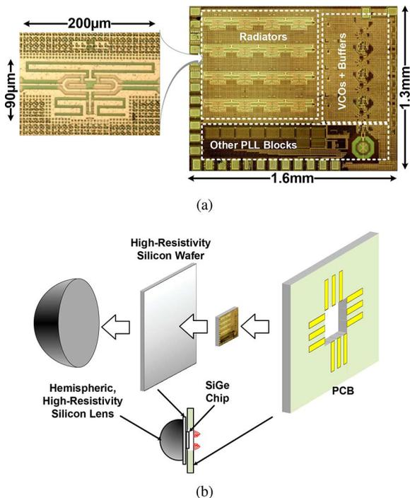
Fig. 18. (a) The microphotograph of the 320 GHz transmitter using 130-nm SiGe BiCMOS process. The THz radiator based on the return-path gap coupler is also shown. (b) The chip packaging with the backside attachment of a silicon lens.
