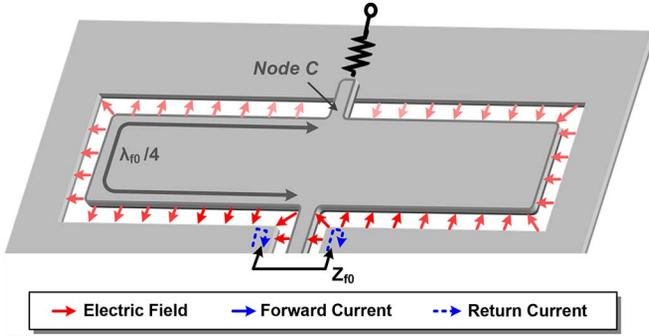
Fig. 7. The standing-wave distribution for the odd-mode oscillation at  $f_0$  in the top slots.
