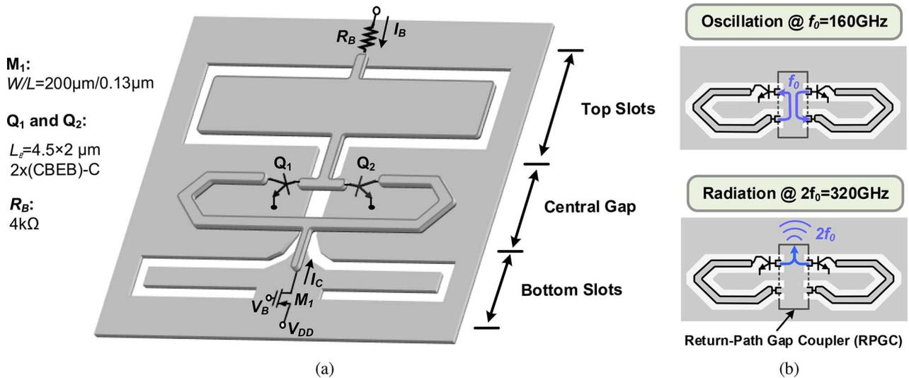
Fig. 5. Proposed THz radiator design: (a) the full schematic and the electromagnetic-wave structure, and (b) summarized operations for fundamental oscillation and 2nd-harmonic radiation. Please note that the structure is not drawn to scale.
