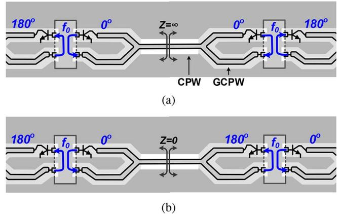
Fig. 15. The mutual coupling between adjacent radiators: (a) in-phase coupling mode (supported) and (b) out-of-phase coupling mode (unsupported).
