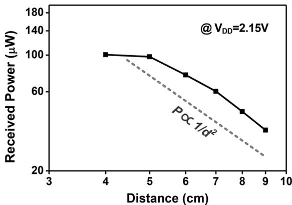
Fig. 21. The received radiated power of the power meter at varying distance,  $d$ , from the 320 GHz transmitter chip.
