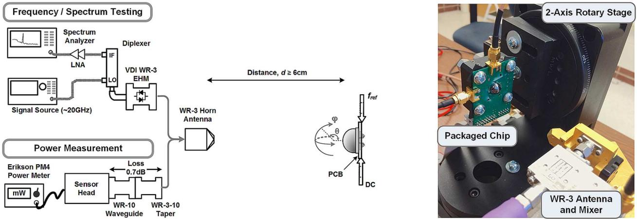
Fig. 19. The measurement setup for the 320 GHz transmitter and a photo of the packaged chip.
