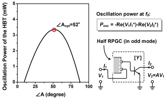
Fig. 11. The two-port active network including a SiGe HBT and a series half-RPGC structure at the transistor base. Also shown is the simulated optimum phase of the complex voltage gain of such active network at 160 GHz.
