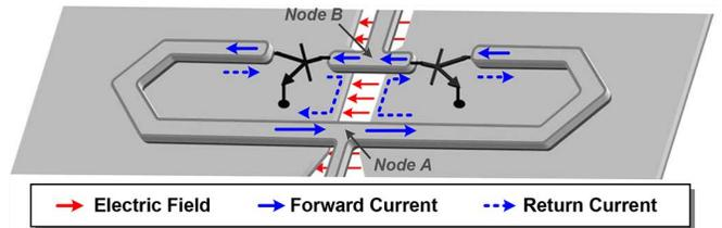
Fig. 6. The current and electric-field distribution for the odd-mode oscillation at  $f_0$  in the central gap.
