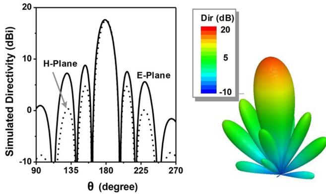
Fig. 16. The simulated radiation pattern of the 320 GHz  $4 \times 4$  radiator array. The pitch between the elements is  $220 \mu\text{m}$ , and a backside hemispheric silicon lens is assumed.
