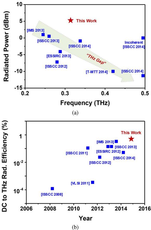
Fig. 1. The performance of the state-of-the-art THz radiator sources in silicon: (a) the total radiated power at varying frequencies and (b) the achieved DC to THz radiation efficiency over the past few years.
