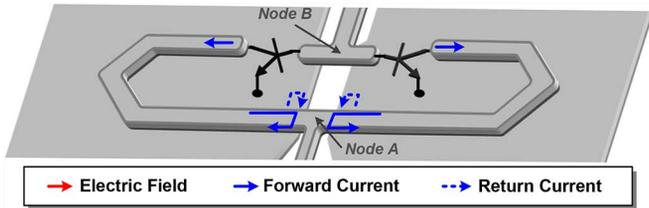
Fig. 8. The current and electric-field distribution for the even-mode oscillation at  $f_0$  in the central gap.
