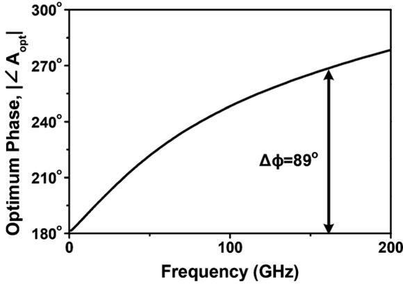
Fig. 2. The simulated optimum phase of the complex voltage gain for a 130 nm SiGe HBT ( $L_c = 4.5 \times 2 \mu\text{m}$ ). Please note that the phase of  $A_{\text{opt}}$  is negative, representing the physical delay from the input to the output of a transistor.
