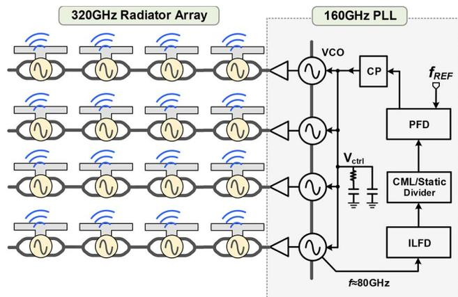
Fig. 14. The architecture of the 320 GHz transmitter with a fully-integrated phase-locking loop (CP: charge pump, PFD: phase/frequency detector, CML: current-mode logic, and ILFD: injection-locking frequency divider).
