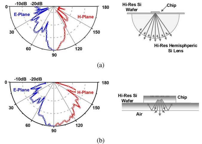
Fig. 22. The measured radiation patterns of the 320 GHz transmitter (a) with a hemispheric silicon lens attached at the back of the chip, (b) direct backside radiation without a silicon lens.
