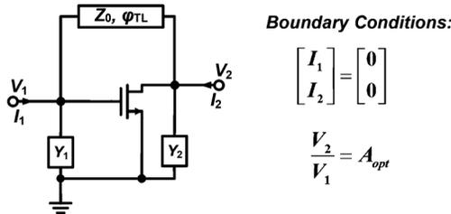
Fig. 3. The simplified schematic of the self-feeding oscillator proposed in [13]. For a self-sustaining oscillator with optimum transistor voltage gain  $A_{\text{opt}}$ , the boundary conditions shown in the figure are required and lead to the relation derived in (1).
