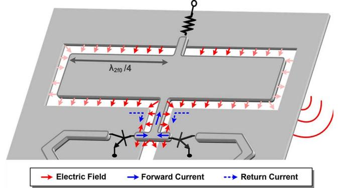
Fig. 9. The standing-wave distribution for the even-mode harmonic signal at  $2f_0$  in the top slots.
