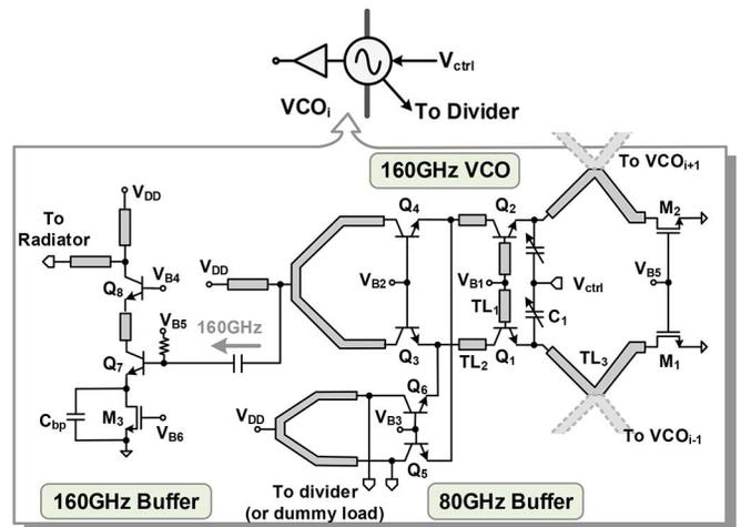
Fig. 17. The schematic of the 160 GHz VCO inside the on-chip phase-locked loop.
