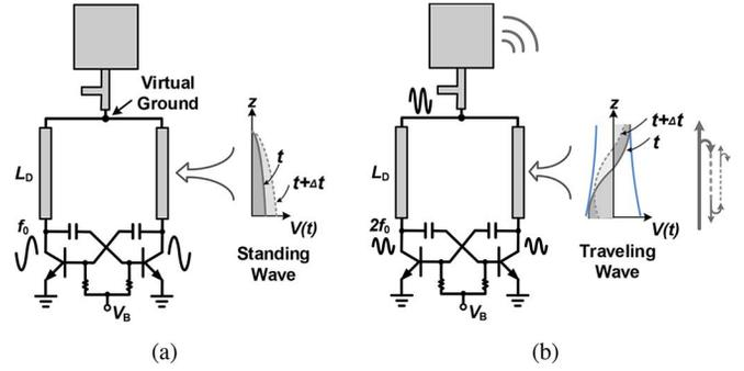
Fig. 4. A typical push-push oscillator: (a) differential standing-wave oscillation inside the near quarter-wavelength-long resonator, and (b) common-mode 2nd-harmonic signal extraction in the form of traveling wave with internal multi reflections.
