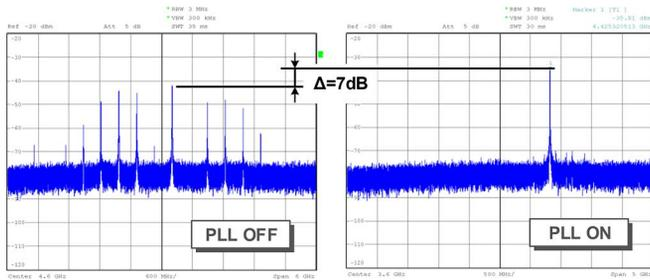
Fig. 20. The measured down-converted spectrum of the transmitter radiation: (a) on-chip PLL is OFF and (b) on-chip PLL is ON.
