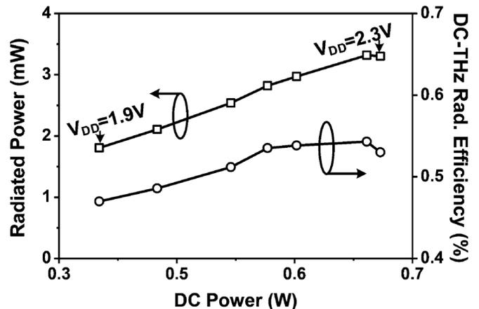
Fig. 23. The total radiated power of the 320 GHz transmitter, as well as the associated DC-to-THz radiation efficiency, at different DC power supply voltage and dissipation power.
