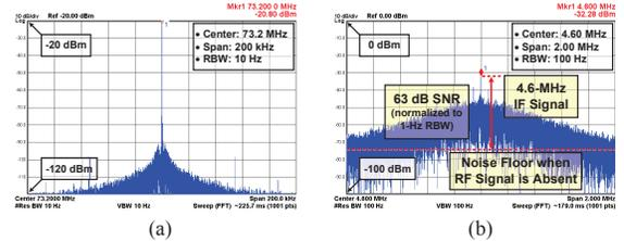
Fig. 6. Spectrum of (a) the output from on-chip divider chain (locked at  $f_{LO}/3200$ ) with  $\text{RBW} = 10$  Hz, and (b) the IF of a unit (Row 1, Col. 2) with  $\text{RBW} = 100$  Hz.
