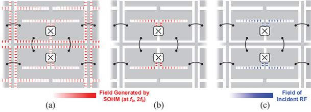
Fig. 3. E-field distribution of (a) generated waves at  $f_0$ , (b) generated waves at  $2f_0$ , and (c) incident RF waves ( $f_{RF} \approx 2f_0$ ).
