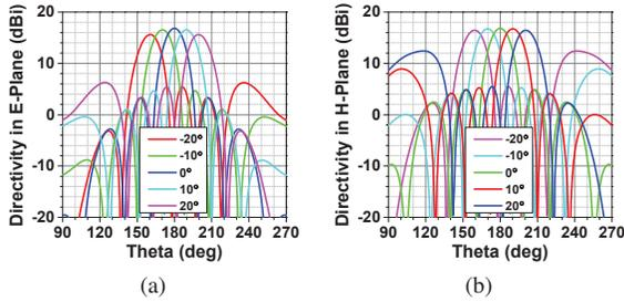
Fig. 4. Simulated beam-steering patterns of a  $4 \times 4$  sub-array in (a) the E-plane and (b) the H-plane.
