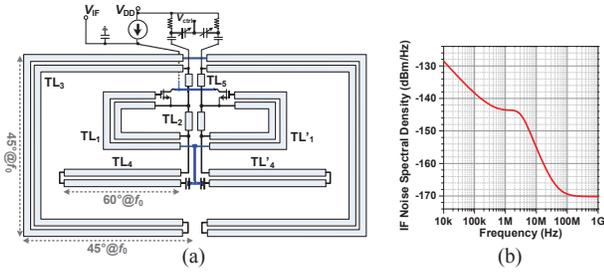
Fig. 2. (a) The equivalent circuit of a single self-oscillating mixer unit. All fixed capacitors behave as short paths for the signals at  $f_0$  and  $2f_0$  (open for  $V_{IF}$ ). (b) Simulated noise spectral density at the IF output with a 50- $\Omega$  load.
