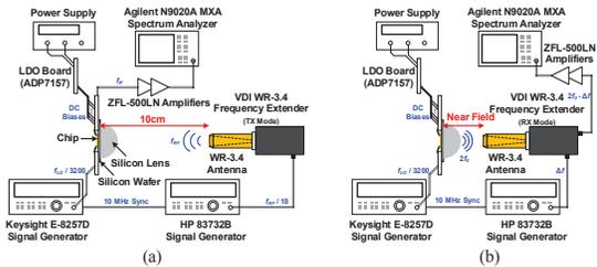
Fig. 7. Setups for testing (a) IF signal, (b) leaked LO at  $2f_0$ .
