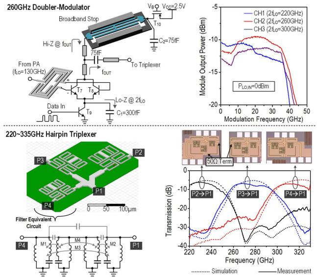
Figure 11.9.2: (Top) design of the 260GHz doubler-modulator, and (bottom) the design, simulation and measurement of the 220~335GHz hairpin triplexer.
