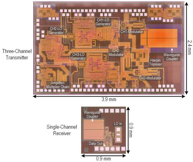
Figure 11.9.7: Die micrographs of the 3-channel transmitter and the single-channel receiver.
