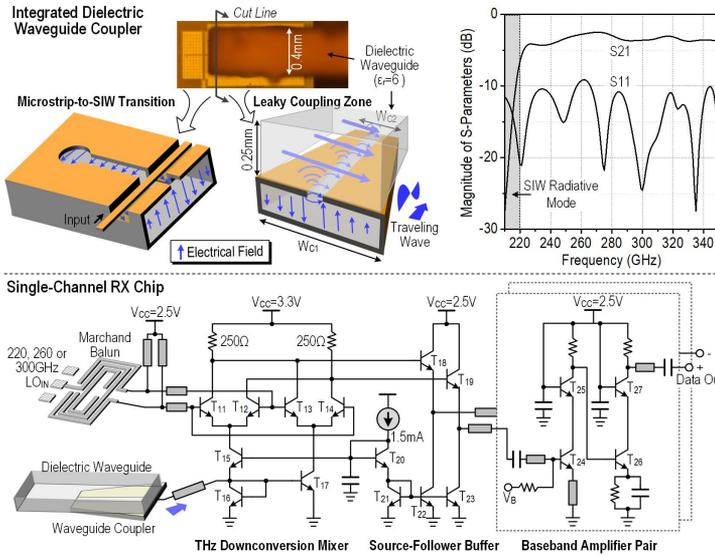
Figure 11.9.3: (Top) the integrated waveguide coupler and simulation results. (Bottom) schematic of the coupler-integrated, single-channel link receiver.
