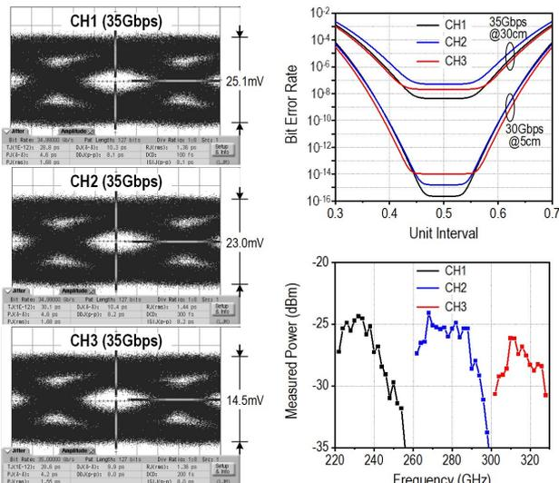
Figure 11.9.5: (Left) measured eye diagram of the 30cm link with an aggregated data rate of 3x35Gb/s, (top right) the measured BER, and (bottom right) the measured output power of each channel.
