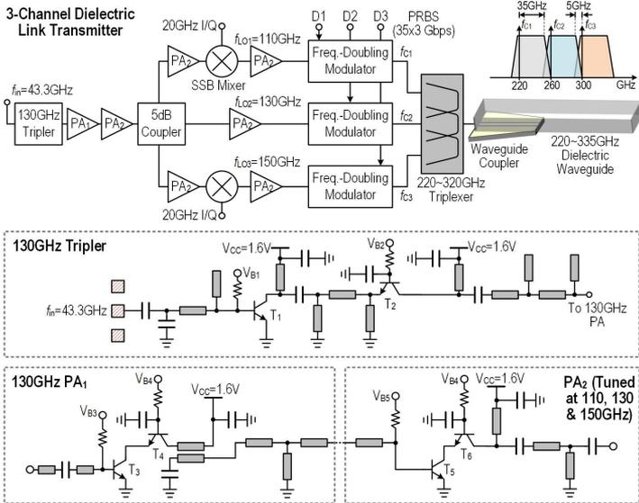
Figure 11.9.1: (Top) system diagram and (bottom) the multiplier and amplifier chain for LO generation.
