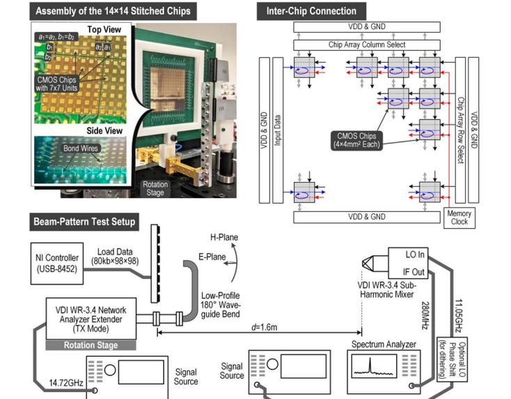
Figure 4.5.4: (Top) assembly and inter-chip connection of the chip array. (Bottom) setup for the beam-pattern measurement.
