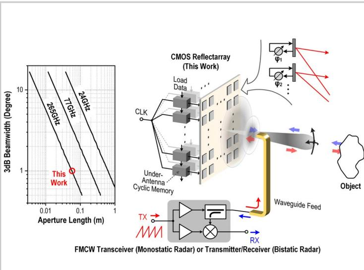
Figure 4.5.1: (Left) Tradeoff between aperture size and beamwidth of beam forming, (Right) architecture and operation of the presented 265GHz CMOS reflectarray.
