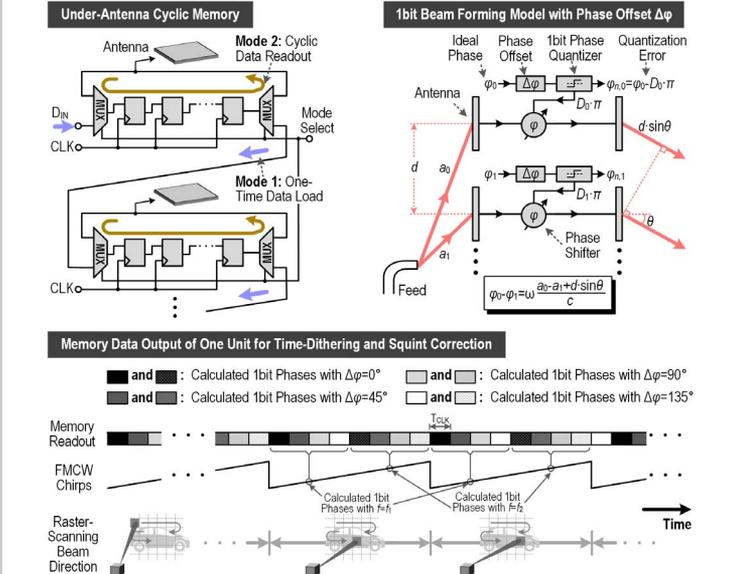
Figure 4.5.3: Sidelobe reduction and squint correction enabled by the under-antenna integrated memory cells.
