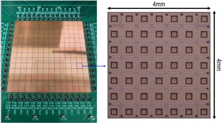
Figure 4.5.7: Photos of the CMOS chip and the array assembly.
