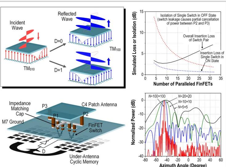
Figure 4.5.2: (Left) Design of the memory-integrated reflect antenna and the 1-bit phase-shifting operation; (Right) simulated performance and the beam-forming patterns of various 1-bit reflectarray sizes,  $N$ .
