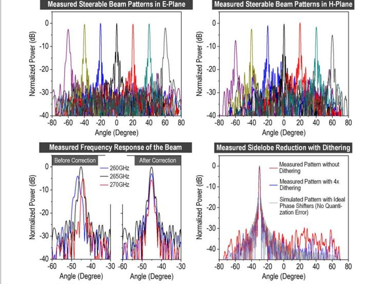
Figure 4.5.5: (Top) Measured radiation patterns of electronically-scanned pencil-beam steering in both E and H-planes. (Bottom) Demonstration of algorithms for beam-squint correction and sidelobe mitigation.
