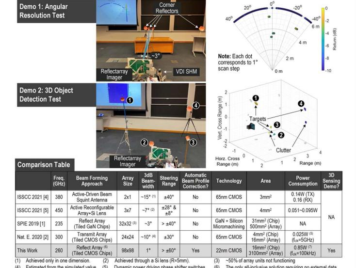
Figure 4.5.6: (Top) Imaging demonstration. (Bottom) comparison with the state-of-the-art THz beam-forming chips.
